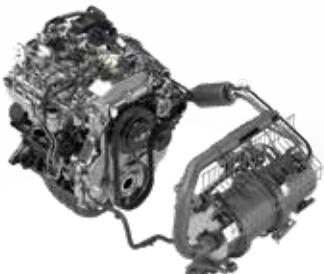
This 3-cylinder industrial diesel engine is mounted in the 2.0 to 3.5 tonne diesel M300. It has a chain-driven distribution and delivers very high torque even at low engine speed thanks to the variable nozzle turbo charger.
